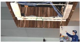
Displaying virtual excavations to facilitate building maintenance.
