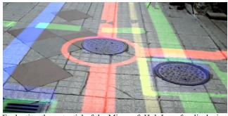
Evaluating the potential of the Microsoft HoloLens for displaying vertical projection of subsurface utility pipes on the road surface.
